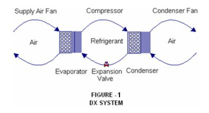
In this schematic, the heat is extracted from the space and expelled to the outdoors (left to right) through 3 loops of heat transfer.
