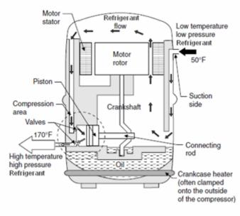
FIGURE - 7 CROSS SECTION OF HERMETIC COMPRESSOR
