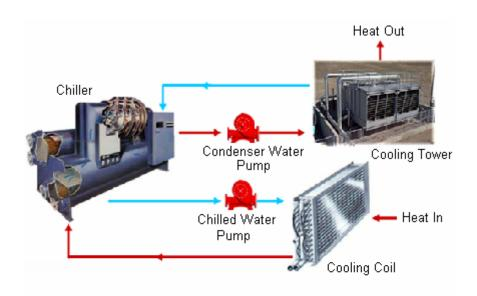
FIGURE - 4 CHILLED WATER SYSTEM
